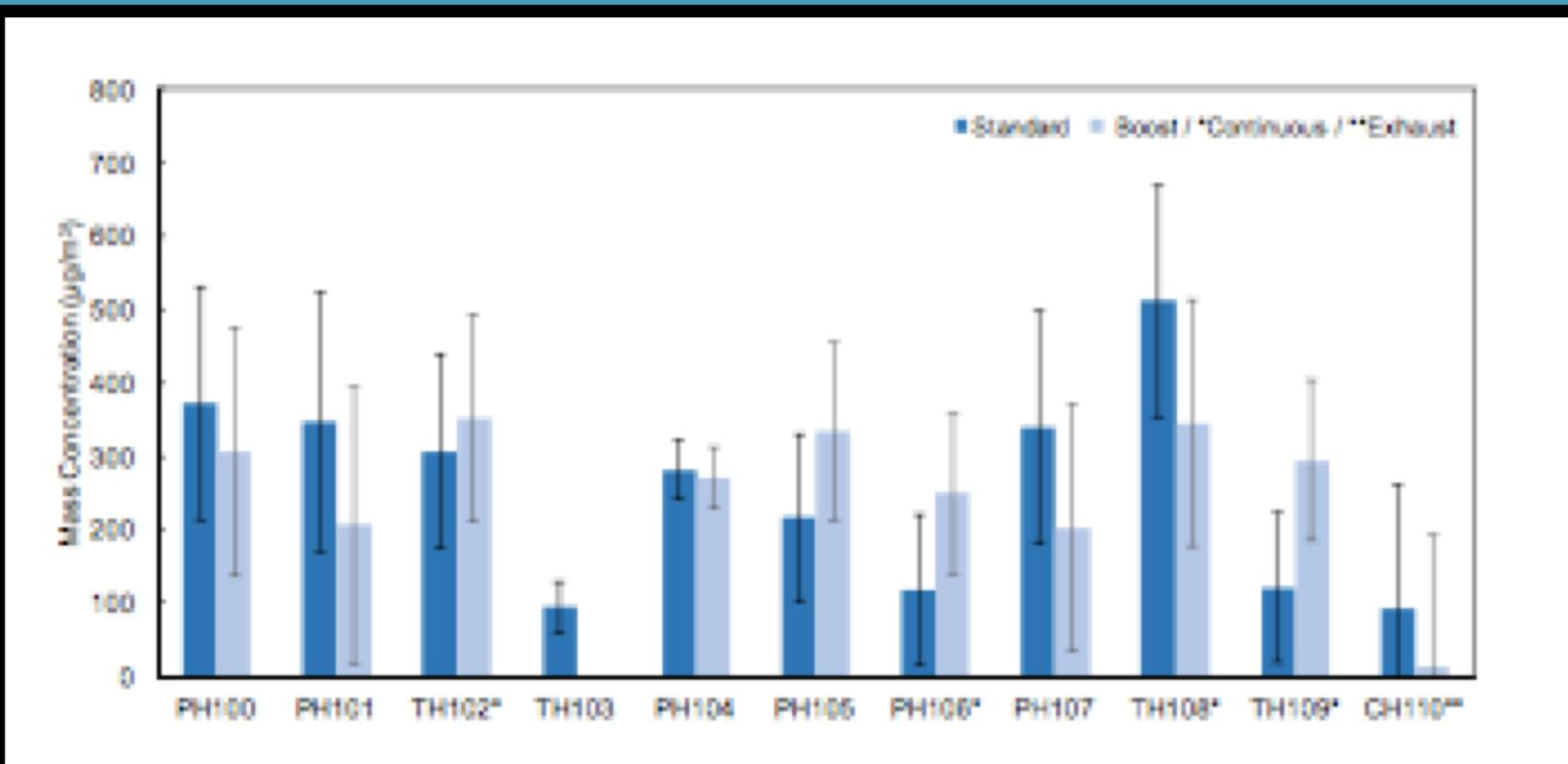
Figure 1. Short-term (20 or 30 minute) PM<sub>2.5</sub> average concentration after cooking for under each ventilation modes. Boost and Exhaust ventilators ran for 20 minutes, Continuous mode ventilators ran for 30 minutes. Bars represent a 95% confidence interval for concentration averages in each ventilation mode.
