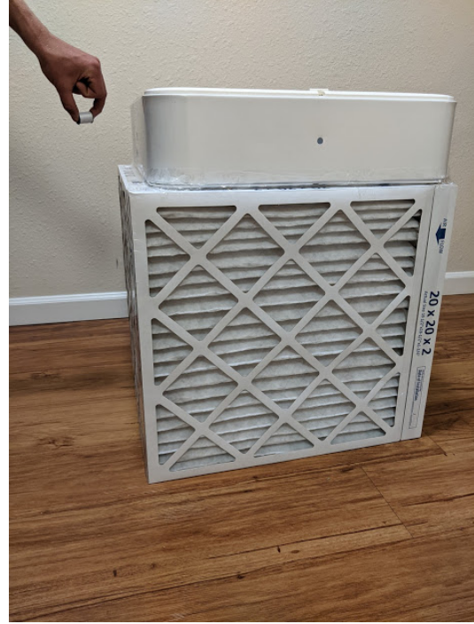
Figure 1: Photos of constructed DIY air cleaner and testing air flow around filters and seams.
