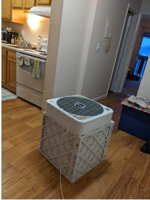
Figure 1: Photos of constructed DIY air cleaner and testing air flow around filters and seams.
